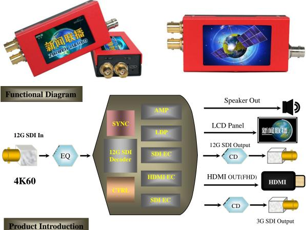
DeviceWell K grade signal converter, a 4K signal conversion device based on broadcast single-link 12G SDI signal. This device input supports up to single-link 12G
